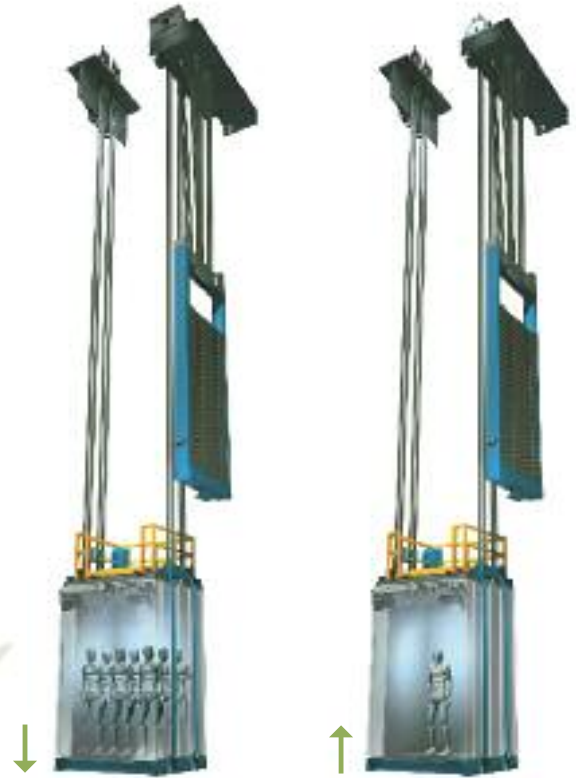
Heavily-loaded car in down direction
